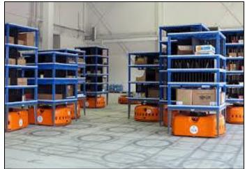
Figure 22: Kiva Systems robots with picking racks
